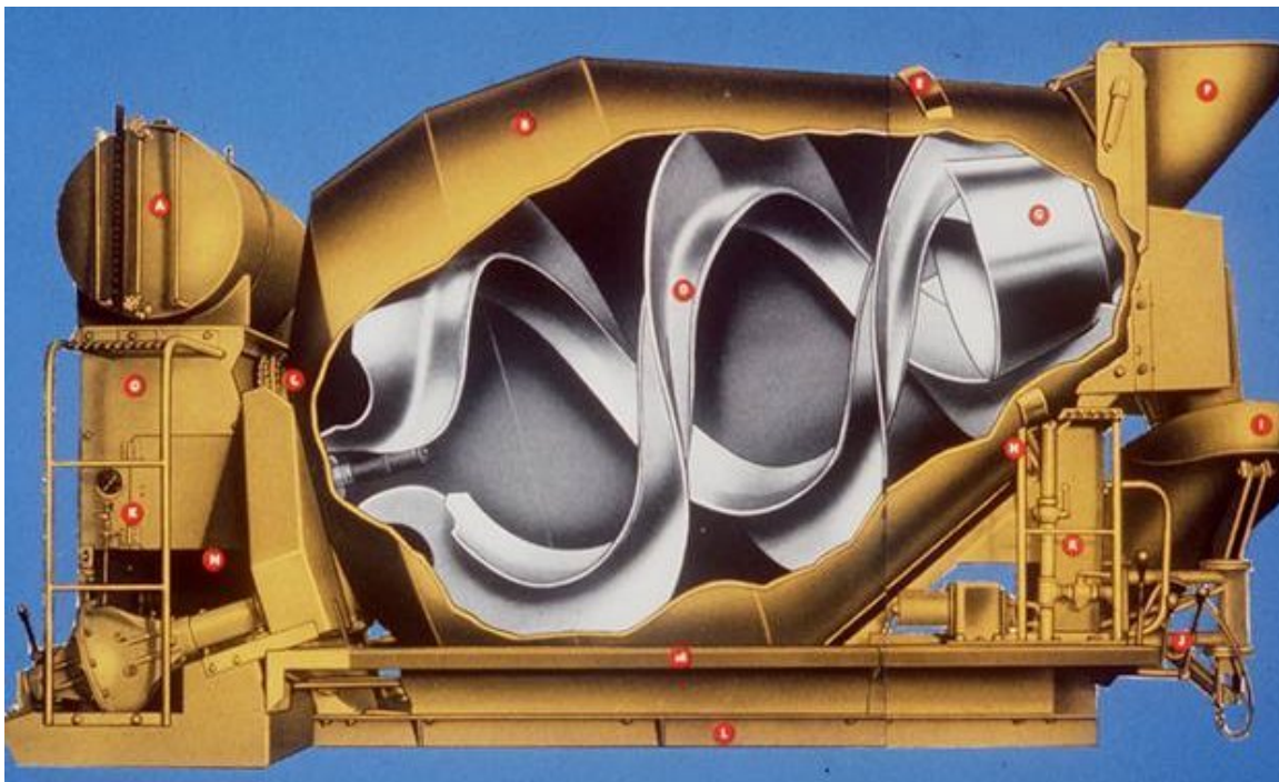
Figure 4-13 Cut-Away View of Transit Mix Drum
