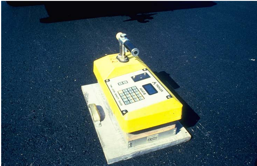
Figure 3-49 Density Measurement with Density Gage
