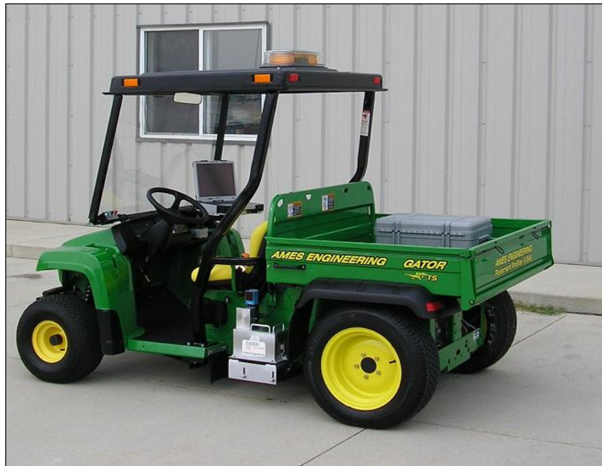
Figure 4-124 Inertial Profiler (“LISA,” Manufactured by Ames Engineering)
