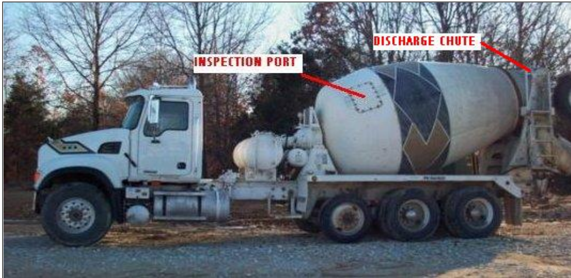
Figure 4-16 Inspection Port on Inclined-Axis Revolving Drum
