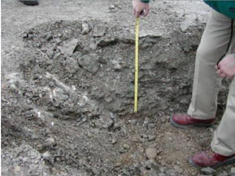
Figure 4-34 Resonant Rubblized Section
